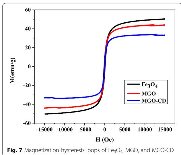
**Fig. 7** Magnetization hysteresis loops of  $\text{Fe}_3\text{O}_4$ , MGO, and MGO-CD
