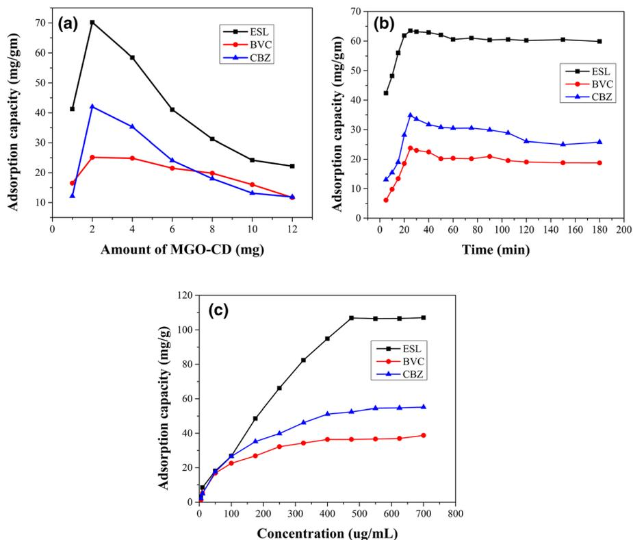
**Fig. 3** a Adsorption capacity of MGO-CD. b The study of adsorption kinetics. c The study of adsorption isotherm
