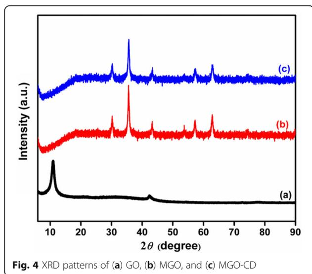
**Fig. 4** XRD patterns of (a) GO, (b) MGO, and (c) MGO-CD
