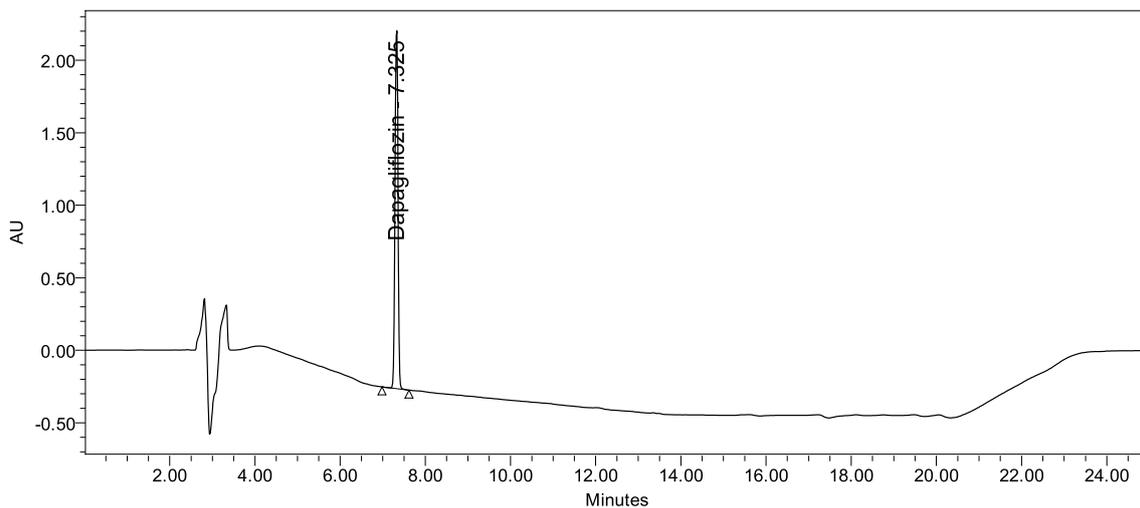
**Fig. 6** Chromatogram for thermal degradation
