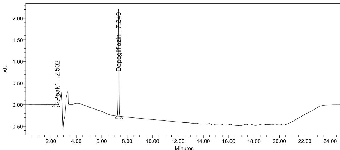
**Fig. 3** Chromatogram for base degradation
