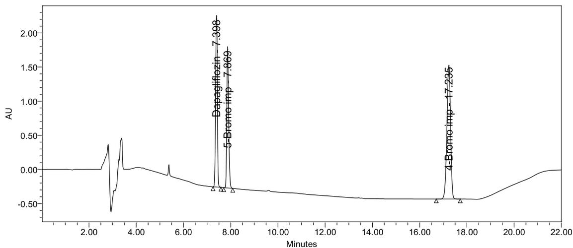
**Fig. 1** Typical chromatogram of DFP, 5-BC impurity, and 4-BC impurity
