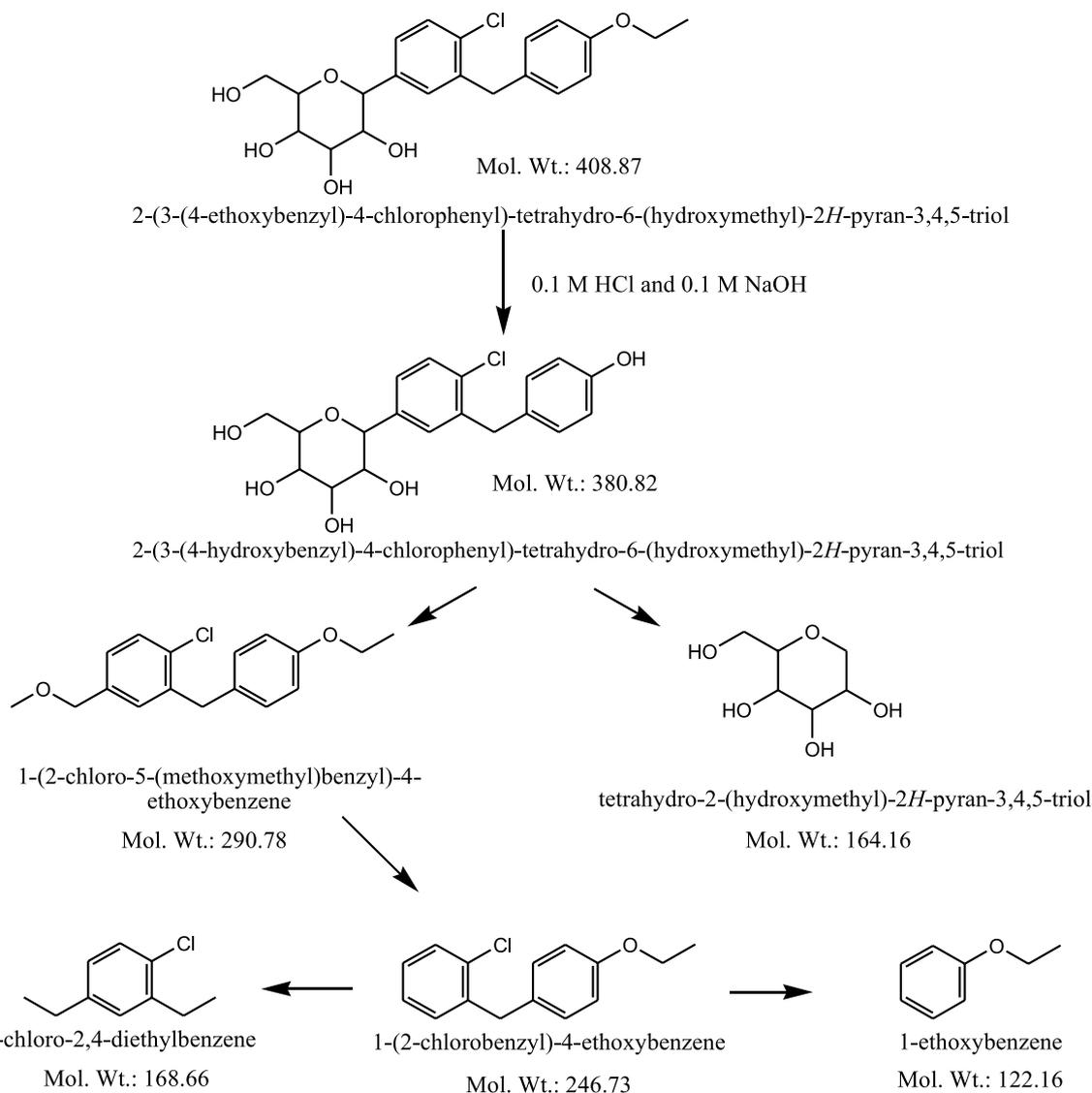
**Fig. 8** The suggested fragmentation paths of DPF degradation products under acid and base hydrolysis
